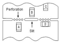
(3) Mounting components near screw holes
